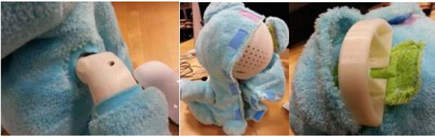
**Figure 6. Huggable's fur pieces can be removed and washed for infection control at the hospital.**
