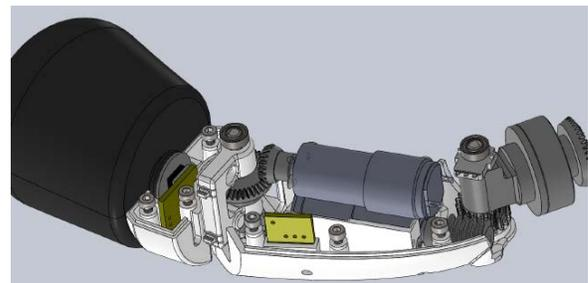
**Figure 5. The pressure bladder is attached to the arm with two pins and can be easily replaced with a new sensor.**
