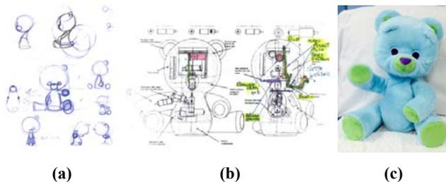
**Figure 1. Huggable's design process started from a professional animator's (a) character sketches, (b) mechanical designs and to (c) the final product as a robot platform.**
