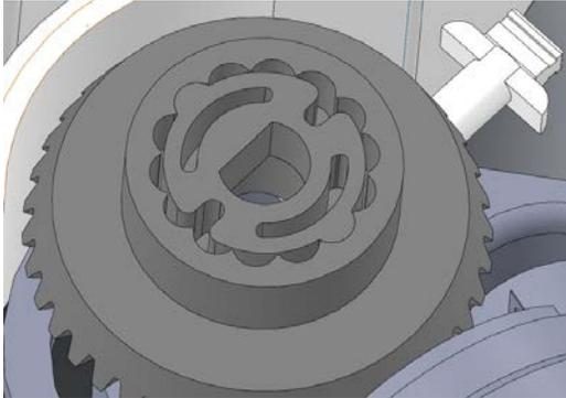
**Figure 3. A flexure clutch mechanism was installed in arm joints to prevent gears from being damaged.**
