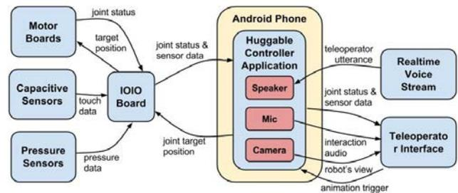
**Figure 2. External sensory data and motor control information are sent to the Huggable controller application on the Android smart phone via IOIO board, and the controller application utilizes the internal phone sensors and features to communicate with the teleoperation interface.**
