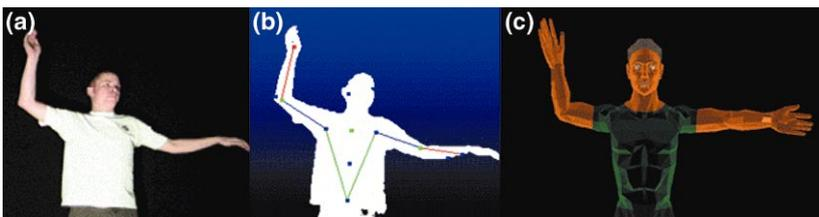
**Fig. 3.** *Adonis*, a rich physics-based simulation of a humanoid upper torso, which has learned to dance the Macarena based on motion capture data from a human dancer. *Adonis* uses motion primitives to map the recorded movements of the human dancer to the range of possible motions that it is capable of performing.
