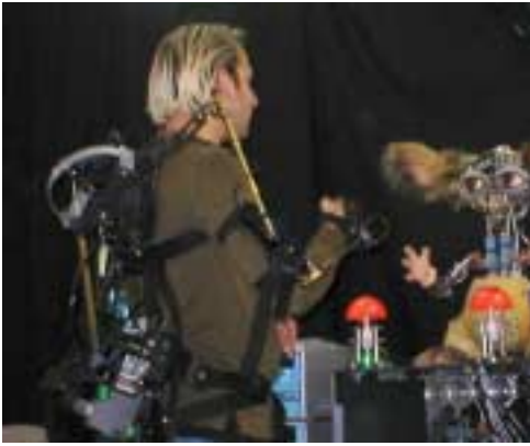
Figure 7: A motion capture suit captures human body poses which the robot must learn to relate according to its own body structure.
