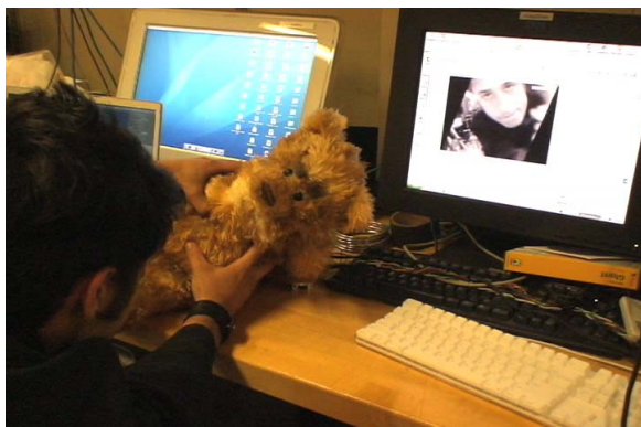
Fig. 3. The IMU Stabilization of the Video Stream. As shown in the figure, the robot is being rolled to its side, yet the image of the face on the screen remains relatively upright because of the counter-rotation. The space where no image data is available (because of the counter-rotation) is filled in with black.
