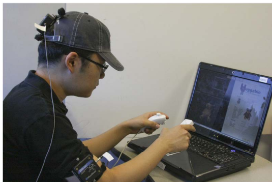
Fig 5. The Wearable Interface. The human operator is holding a Wii Remote and a Nunchuk on both hands and wearing a set of orientation sensors on both arms and the head.
