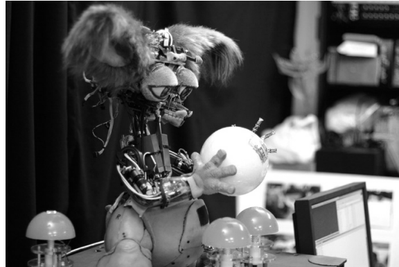
Fig. 3. Leonardo the humanoid robot, possessing 65 degrees of freedom that allow it to interact expressively, as well as perform simple object manipulations. Here Leonardo is surrounded by some of the buttons it uses in object manipulation tasks.
