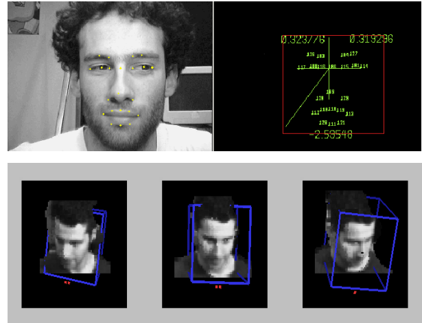
Figure 2: Visual Inputs. Facial feature tracking of 22 nodes (top) and 3D head pose tracking (bottom).
