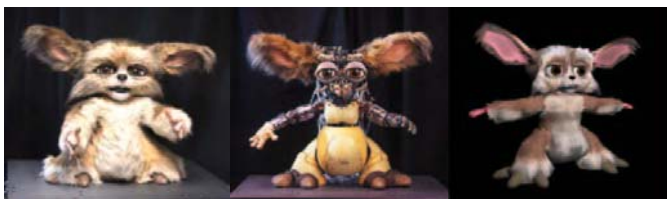
Figure 1: The Leonardo robot when cosmetically finished, the robotic underpinnings, and the simulator. The same cognitive-affective architecture drives both the physical and virtual robot.
