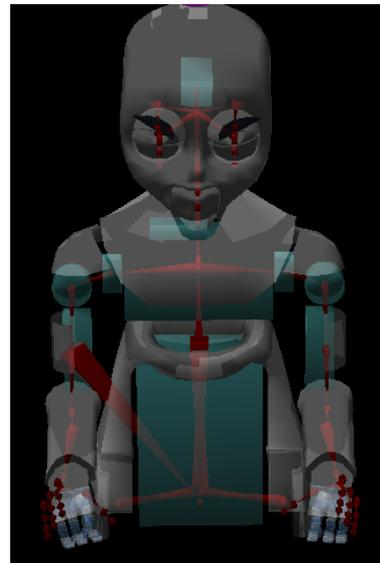
**Figure 3:** A single frame of the “angry” animation blended with the generated speech and visualized in our robot simulator. Clearly visible is the head posture and the characteristic eyebrow location in the robot skeleton (shown in red).
