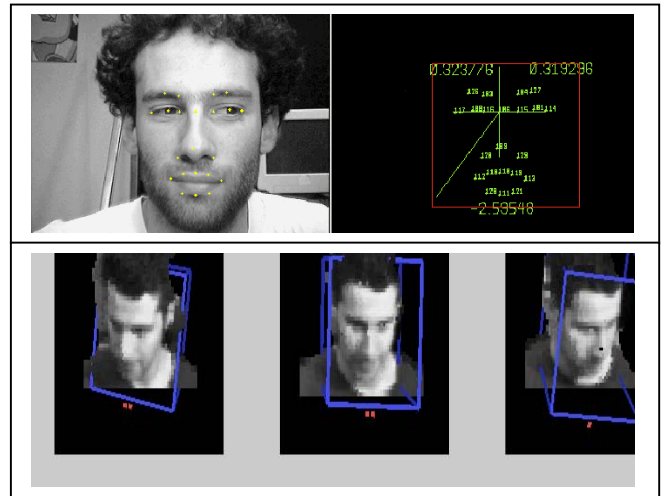
Figure 2: Visual Inputs. Facial feature tracking of 22 nodes (top) and 3D head pose tracking (bottom).
