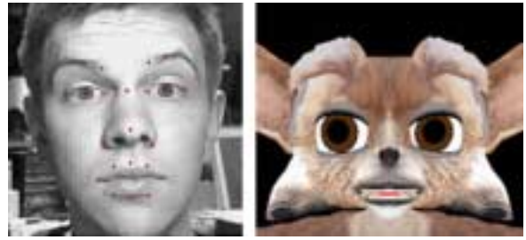
Figure 6: Facial tracking data is captured in real time in the form of the positions of 22 node points, and mapped to the pose space of an animated model of the robot.
