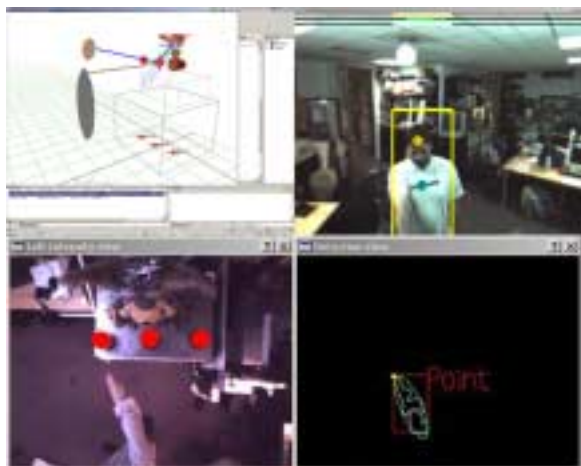
Figure 2: World model representation and human tracking and gesturing output.
