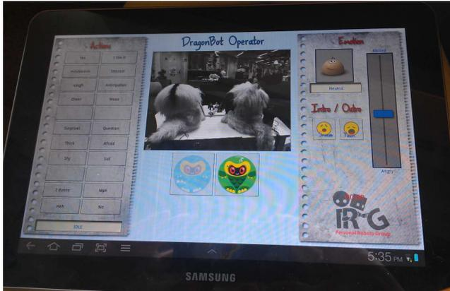
**Figure 2: The tablet-based tele-operation interface for the dragonbot, which allows remote presence interactions.**
