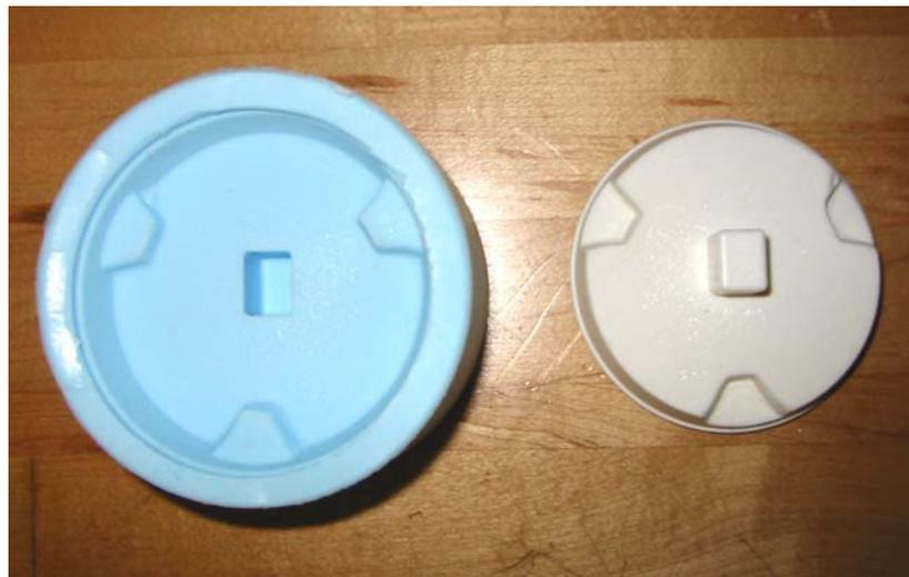
Figure 7-9. The Mold and Cast of the Fingertip Core. The mold (left) used to make the cores (right) features a series of 3 keys which will be used to register the core and the fingertip mold together.
