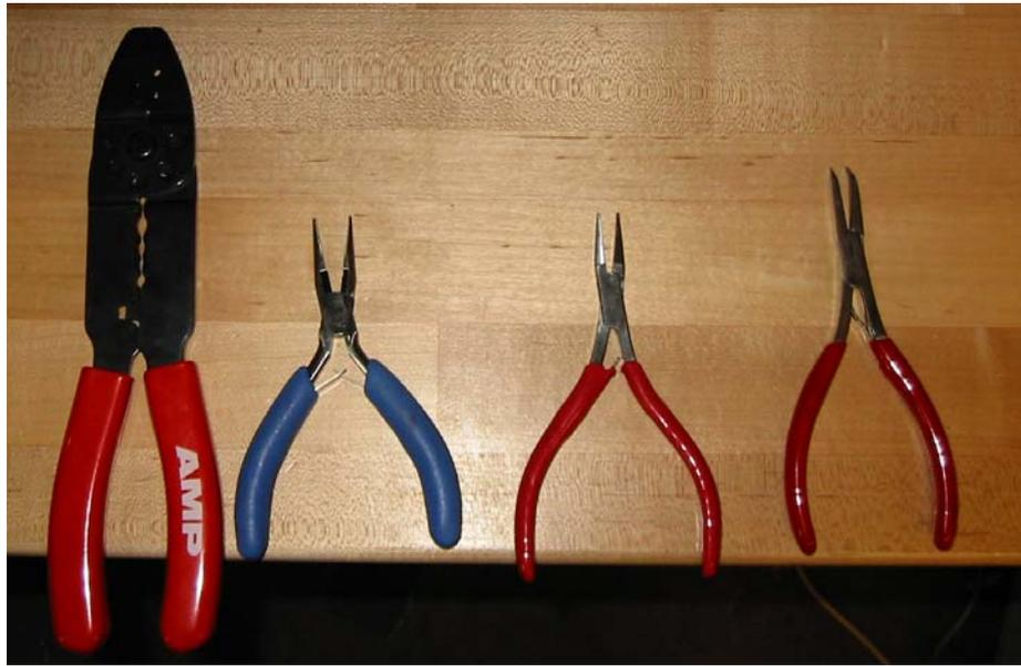
Figure 5- 5. The Four Hand Tools Used to Crimp the Solder Tabs to the Cut FSRs
