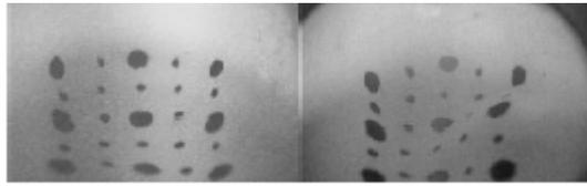
Figure 3-3. Camera View of Membrane: (a) undeformed (b) in contact with object (Hristu, Ferrier et al. 2000).
