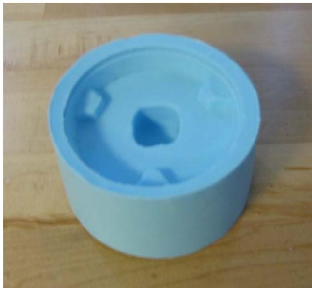
Figure 7-11. The Silicone Fingertip Mold.
